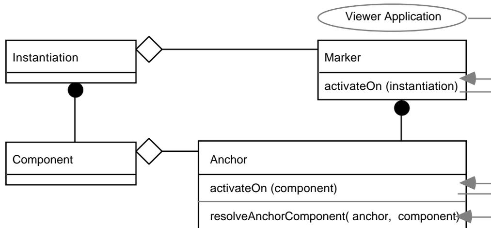
In the above schema, an anchor captures two different aspects of the design, namely the structural reference to a substructure of a component and the way to resolve an anchor-component pair. Mixing two different aspects in a single design element causes difficulties as the design is less configurable and less extensible.
