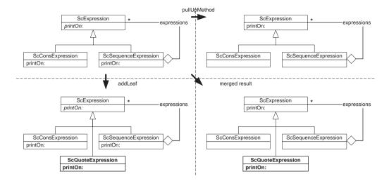
Fig. 1. Applying an addLeaf transformation and a pullUpMethod refactoring in parallel
