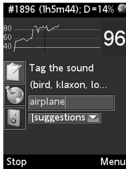
Fig. 4. The NoiseTube Mobile application interface includes the following main components: the measured sound level (visualised with a histogram and a color scale), complemented by a dose indicator (on top), the tagging component and the location tagging component (for indoor locations for instance).
