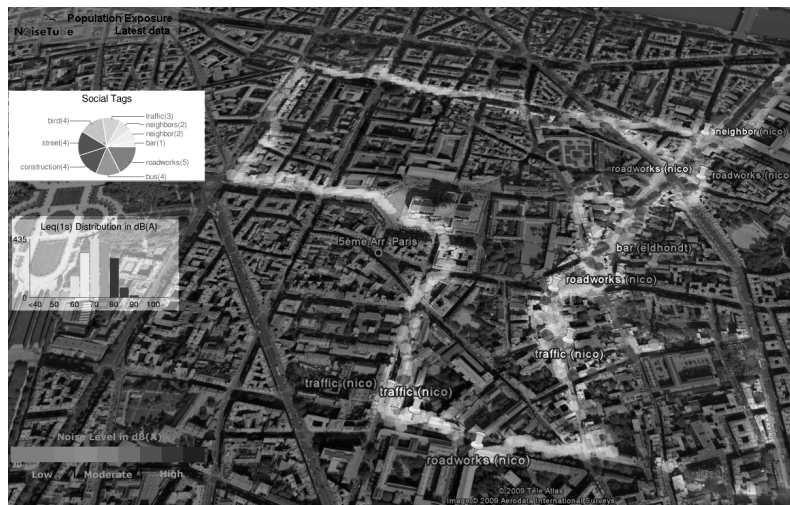
Fig. 9. The collective noise map for Paris, displayed using Google Earth. The legends on the left (pie chart of the social tag cloud and the sound level distribution) are dynamically updated with respect to the area in view.
