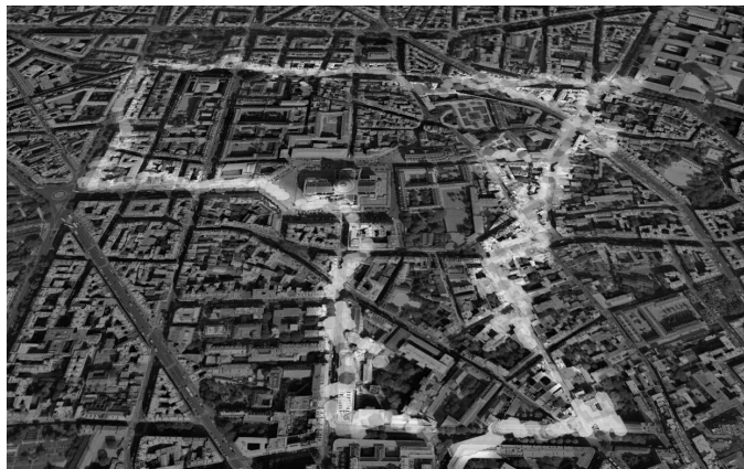
Fig. 10. A noise map of an area of Paris, without applying aggregation.
