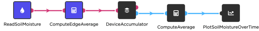
Fig. 17: Flow graph featuring plotting the average soil moisture on a line chart.
