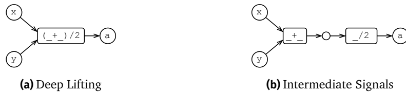
■ Figure 11 Signal graphs that compute the average of two signals. Both a signals are semantically equivalent. Constants have been inlined in these figures for simplicity.
