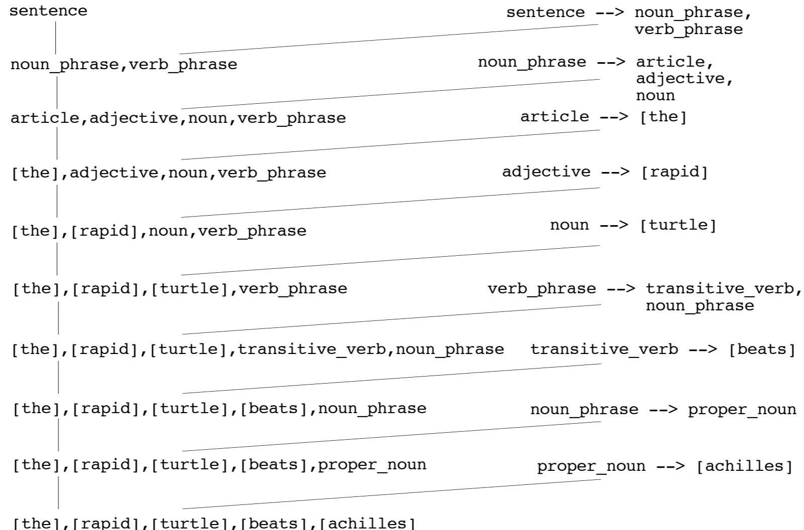
start with NT and repeatedly replace NTS on right-hand side of an applicable rule until sentence is obtained as a list of terminals
