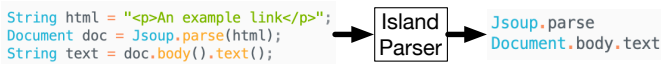
Fig. 4. The API usages extracted by our island parser and its lightweight analysis for the code snippet on the left.
