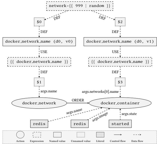
Figure 3: PDG for the defective Ansible role of Figure 1.
