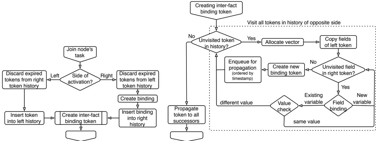
(a) Steps to process incoming tokens of a join node (b) Steps to create infra-fact bindings, i. e., applying unification
